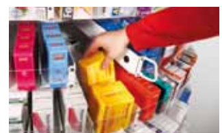
Observance of the FIFO principle thanks to filling from the back
